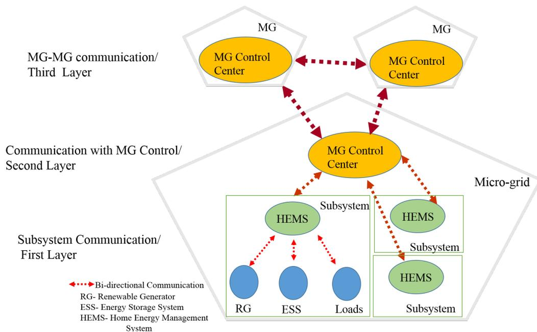
**Figure 1.** Hierarchical communication layers in micro-grid (MG).
